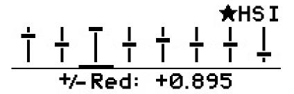
In the upper left and right corner of the display the active special and operation modes are displayed similar to the home screen (in the picture above "HSI" operation mode).
